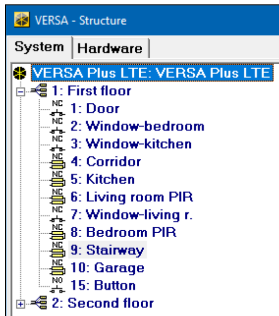
Fig. 6. DLOADX program: list of partitions and zones in a tree-like form in the “System” tab, “VERSA – Structure” window.
